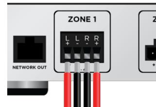
2. Connect all phoenix connectors, auxiliary audio sources, and external audio subsystems.
